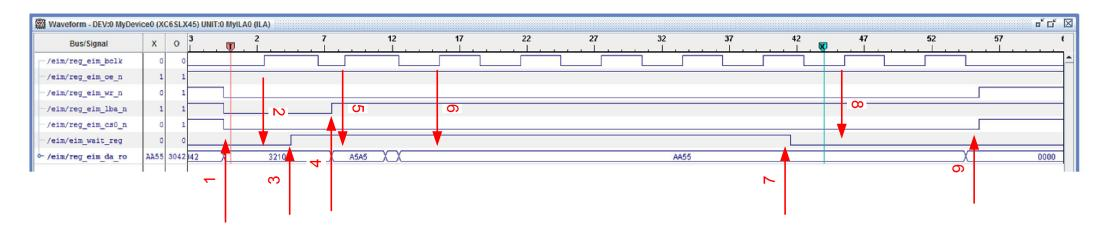
Here is what WRITE transaction looks like. Wait flag is shown using positive logic, it is inverted in actual hardware.
