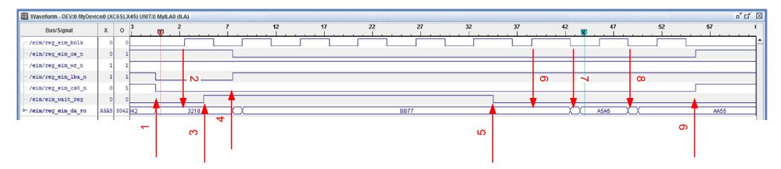
Here is what READ transaction looks like. Wait flag is shown using positive logic, it is inverted in actual hardware.
