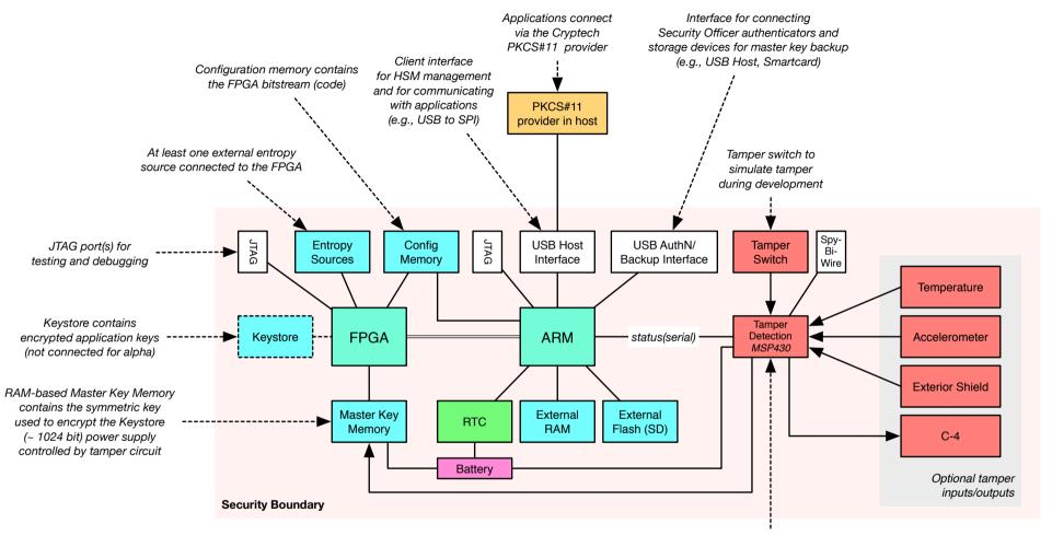
Tamper detection circuit responsible for erasing Master Key Memory upon tamper
