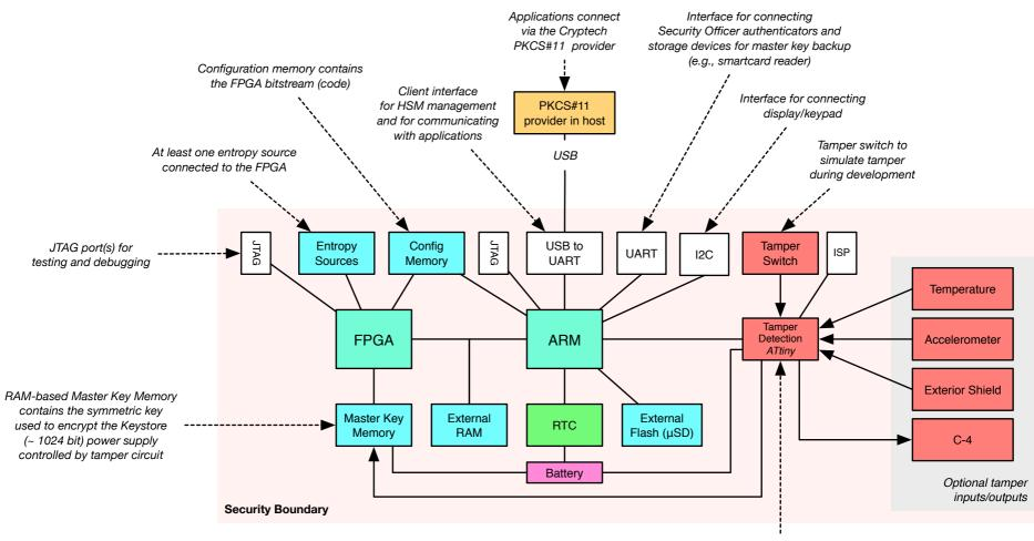
Tamper detection circuit responsible for erasing Master Key Memory upon tamper
